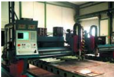
SATRONIK FB/DS with 2 Plasma HyDefinition cutting components
